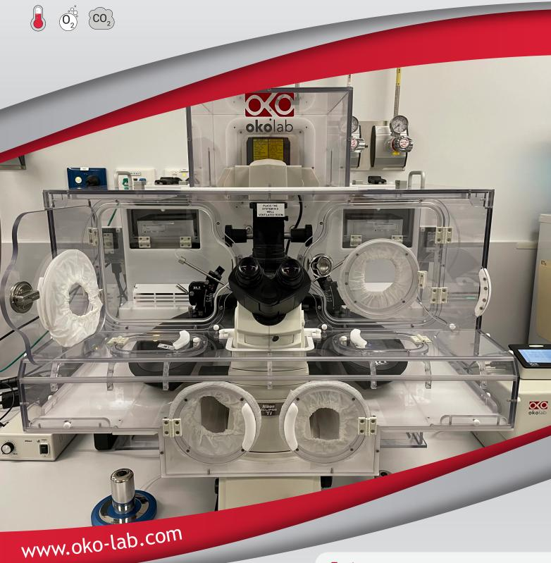
The Okolab ICSI-ENCLOSURE maintains a stable and uniform temperature and CO2/O2 concentrations all around the ICSI workstation.
