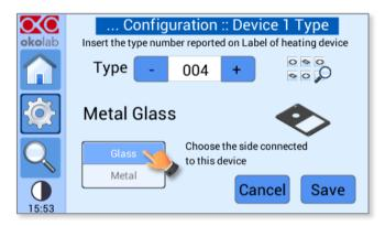
Figure 24. Selection of heating device with glass/metal insert.
