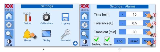
Figure 59. Alarms settings. (a) How to enter the Alarm setting menu; (b) Alarm configuration
