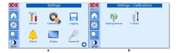
Figure 30. Calibration. (a) How to enter in the calibration menu (b) Calibration menu
