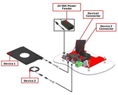
Figure 85. Connection of the heating devices and the power feeder
