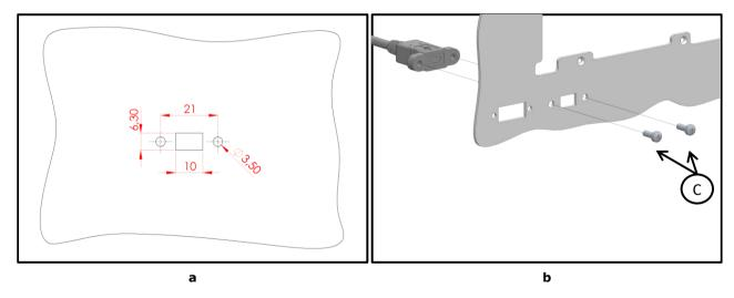
Figure 88. Installation of the Ultra-Thin Mini-B Extension Cable panel. (a) Panel opening size (b) Fixation of the Ultra-Thin Mini-B Extension Cable.
