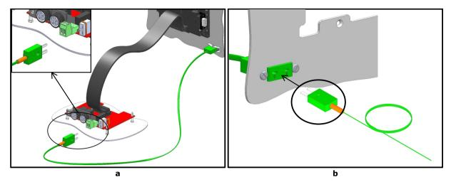
Figure 87. T sensor connection (a) Extension thermocouple cable connection to the control board (b) T sensor connection to the panel
