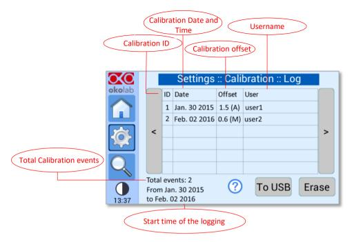
Figure 44. Logging of calibration data
