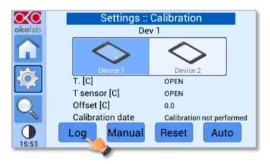
Figure 43. How to recall the stored calibrations
