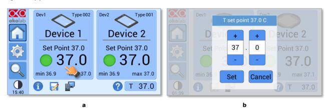
Figure 11. Definition of the set point. (a) Selection of the device; (b) Input of the set point value.
