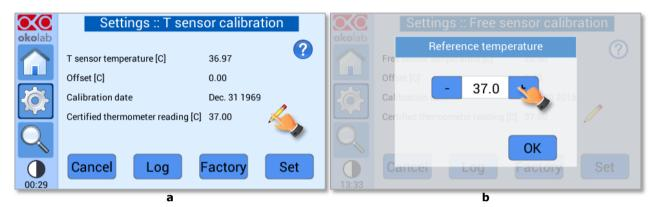
Figure 49. How to re-calibrate the T sensor
