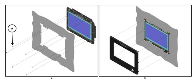
Figure 81. Display installation (a) Display panel mounting; (b) Bezel positioning.
