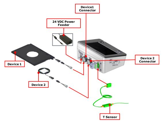
Figure 4. Connection of the heating devices
