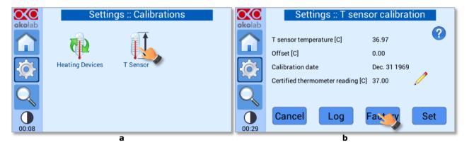
Figure 47. Calibration data. (a) T sensor calibration page selection; (b) T sensor calibration page
