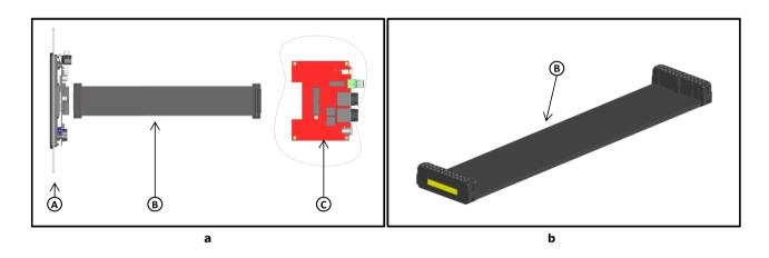
Figure 82. Communication cable (a) Communication cable connections; (b) Communication cable, 3D view.
