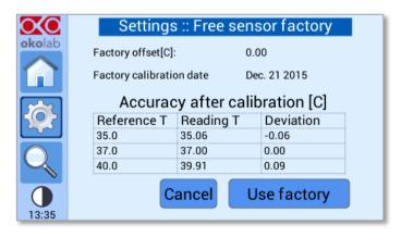
Figure 48. Free sensor factory offset
