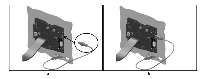
Figure 89. Ultra-Thin Mini-B Extension Cable display connection.
