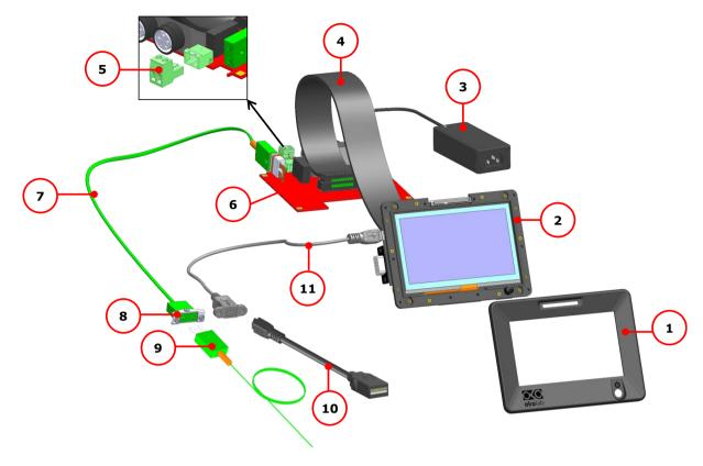
Figure 79.H401-T-CONTROLLER-OEM - Components.
