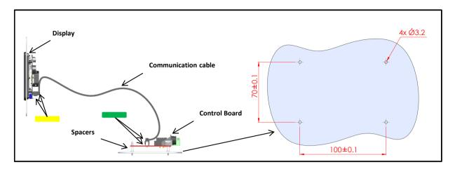
Figure 83. System Lateral View and holes dimensions on the support
