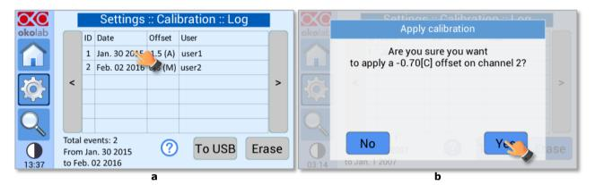
Figure 45. How to apply a previous calibration
