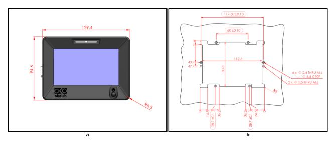
Figure 80. Display and panel opening dimensions. (a) Display size; (b) Panel opening size.
