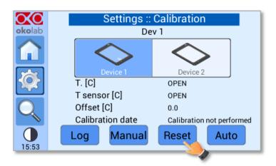
Figure 46. How to reset the offset.
