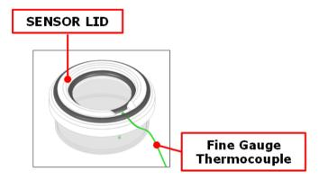
Figure 33. SENSOR LID-35. For 35 mm Petri-dish
